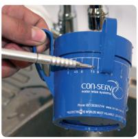
An efficient tap should have a flow rate of less than 9 litres per minute (L/m) and it can be as low as 2 L/m with a very efficient tap. Kitchen and laundry sinks may require flows at the higher end of the scale, while bathroom basins etc. should be towards the lower end.
