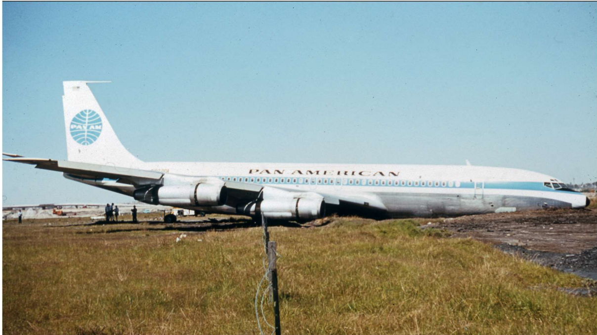
Figure 3. The Pan Am Boeing 707 which overran the end of Runway 34 on 1 December 1969. Despite the extensive damage, air safety investigators confirmed the captain's decision to abort the take-off. Source: Airways Museum. Reproduced with permission.
