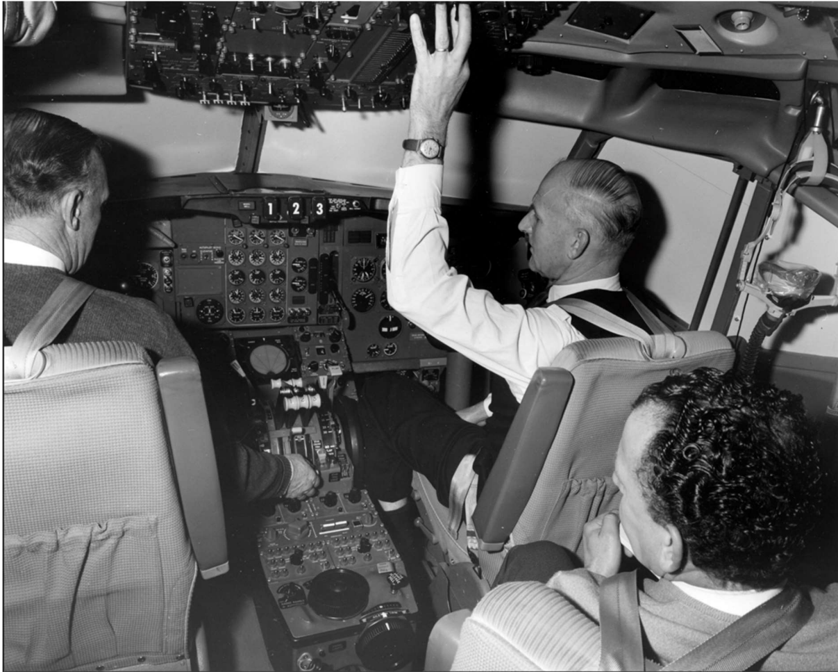
Figure 8. A 1969 photograph of the cockpit of a TAA Boeing 727 flight simulator, illustrating the relative positions of the captain (left), first officer (middle) and flight engineer (right). Source: Airways Museum. Reproduced with permission.
