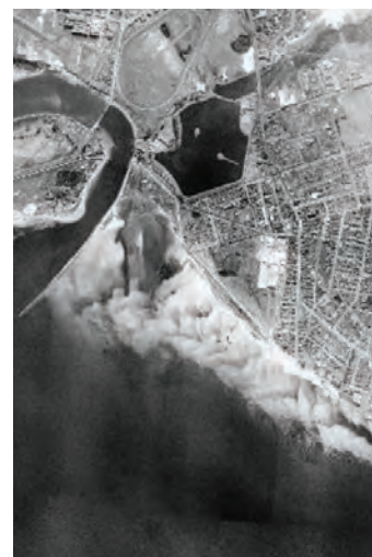
Figure 3.4.6 The 1943 aerial photograph shows how the construction of the sea-wall near Booralee to divert the flow of the Cooks River resulted in major siltation of the bay adjacent to the village with subsequent destruction of the local fishing industry. (NSW LPI SLX maps)
