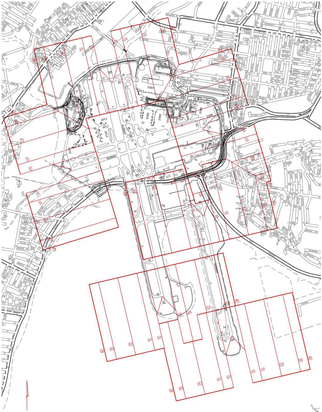
Figure 1: NASAG zones showing minimum height limits requiring assessment and OLS relative to AHD
