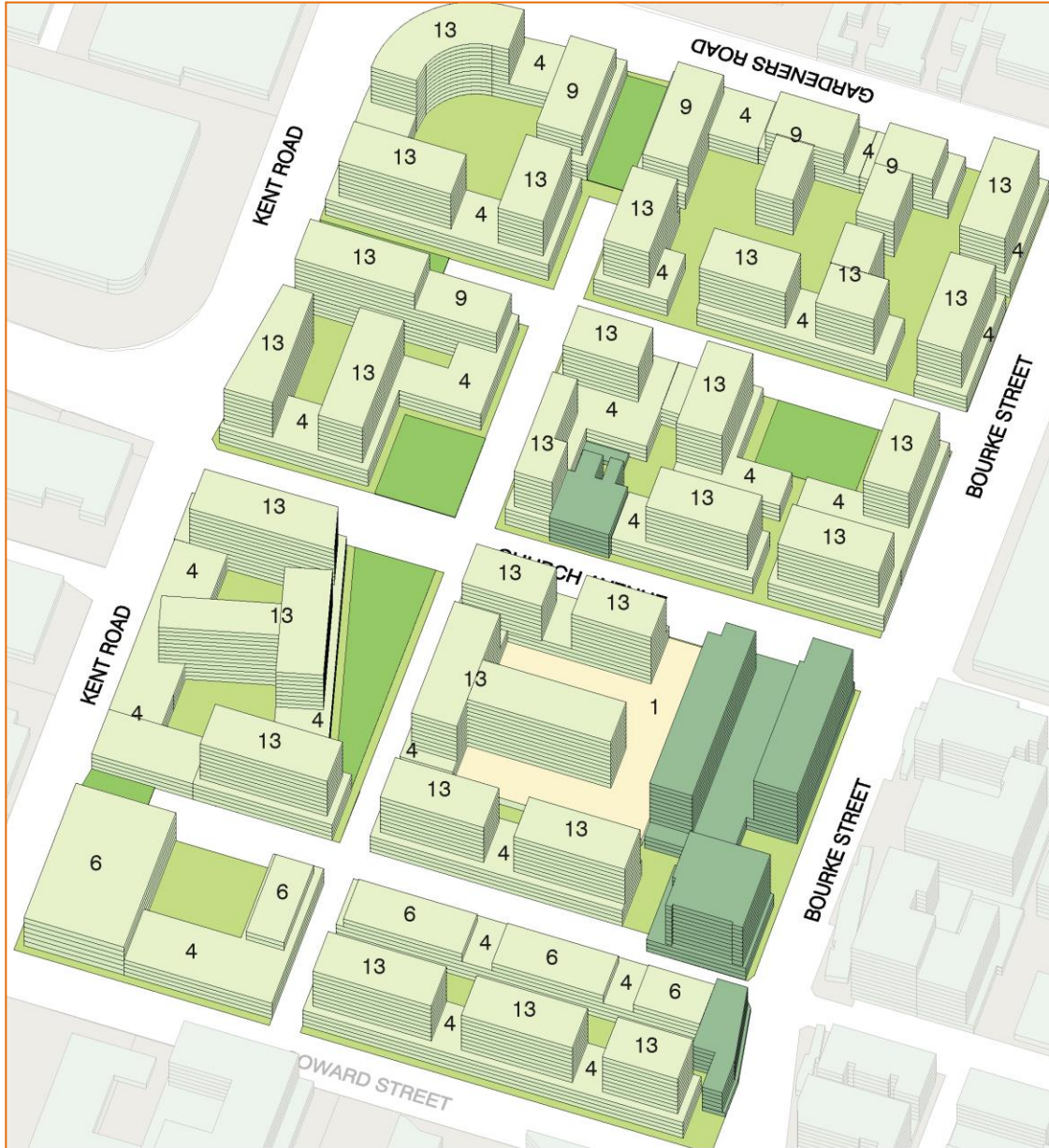
Figure 43 - 3D Building Envelopes - Urban Block 1
