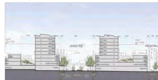
Figure 63: Section of Kingsford Junction showing 17 storey building typology with four storey street wall and mews development at the rear. Source: Conybeare Morrison 2016
