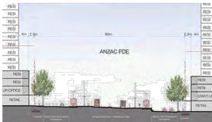
Figure 67: Section showing proposed 1.5m setback adjacent to nine storey building Source: Conybeare Morrison 2016
