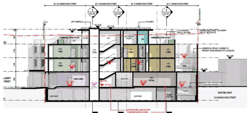
Figure 3 Section Plan CC (Plan Ref: DA-162(I)) demonstrating height non-compliance
