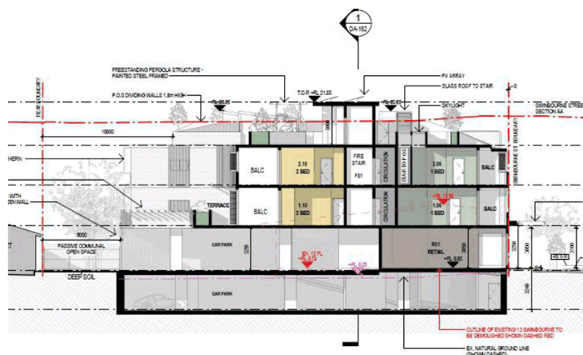
Figure 2 Section Plan AA (Plan Ref: DA160(J)) demonstrating height non-compliance
