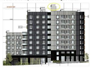
Figure 1: Extract of proposed elevation with height breach outlined yellow (Source: DKO Architects)
