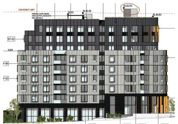
Figure 4 - Extent of building height variation to lift overrun to access rooftop communal open space
