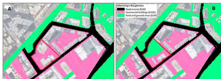
Figure 7 Manning's roughness values used in the models (A) Original WMA model and (B) Revised existing case model
