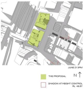
Figure 13: Solar analysis June 21 3pm
