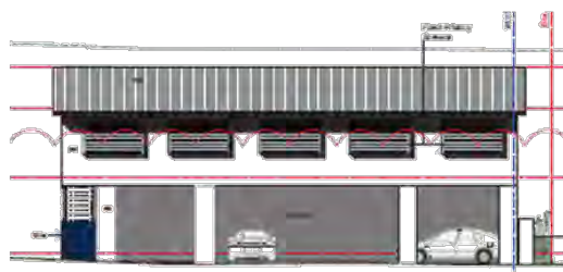
Figure 4: Southern elevation plan showing louvers to first floor boarding rooms
