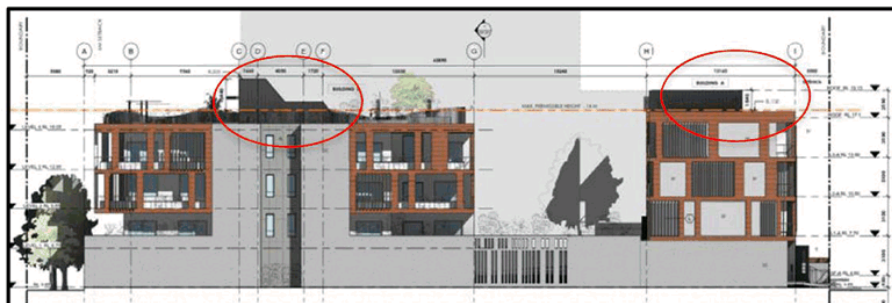
Figure 3: Western elevation extract identifying non-compliant building height
