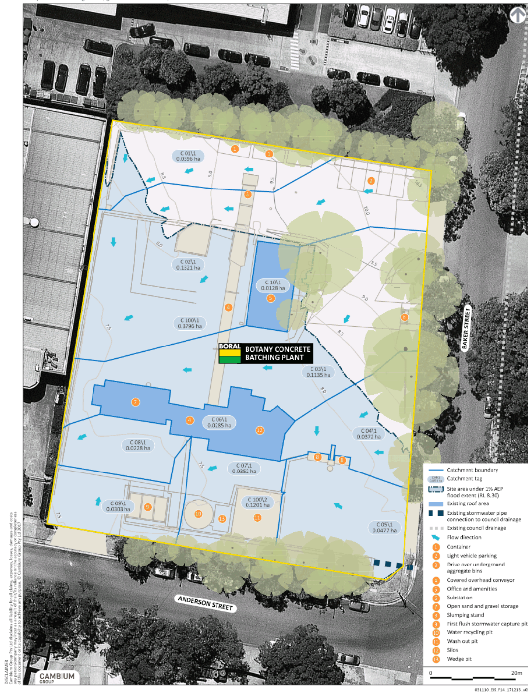
FIGURE 14 EXISTING STORMWATER MANAGEMENT SYSTEM Botany Concrete Batching Plant Upgrade - Environmental Impact Statement
