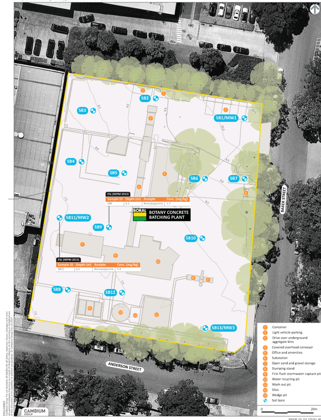
FIGURE 12 SAMPLE EXCEEDANCES OF SOIL ASSESSMENT CRITERIA Botany Concrete Batching Plant Upgrade - Environmental Impact Statement
