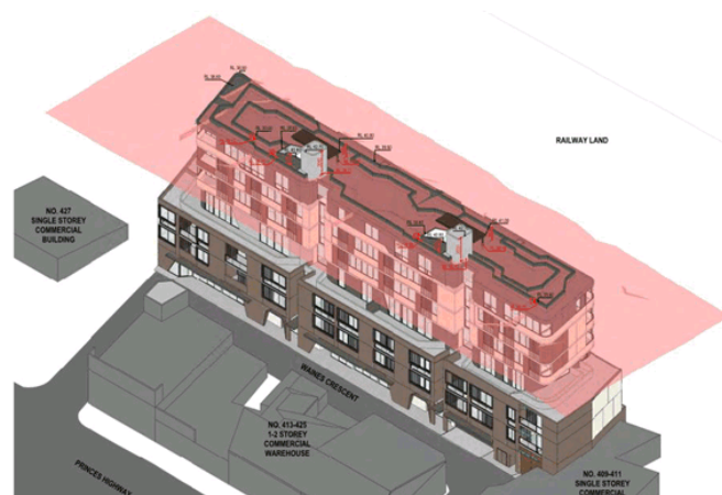
Figure 14. Extract of the RLEP height blanket diagram indicating the RLEP height exceedance (Source: CD Architects).
