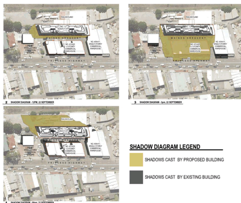
Figure 18. Equinox shadow diagrams at 9am, 12pm and 3pm (Source: CD Architects).
