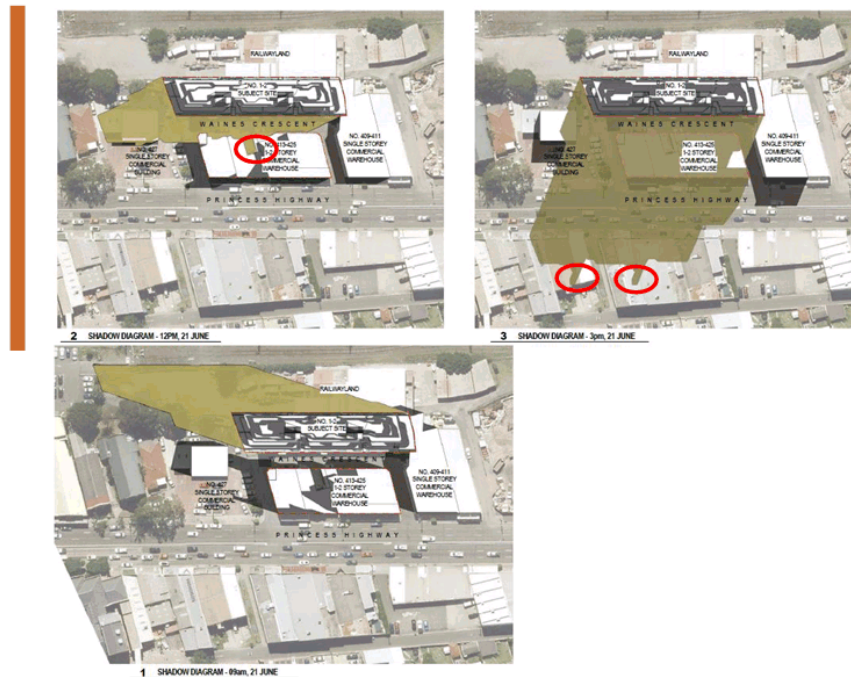
Figure 5 - Overshadowing impact of height variation (circled red)
