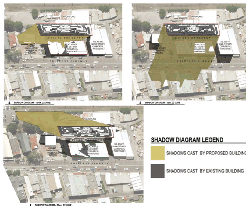
Figure 17. Mid-winter shadow diagrams at 9am, 12pm and 3pm (Source: CD Architects).
