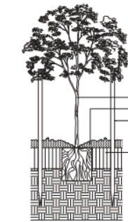
1 HARDWOOD STAKING FOR TREES SCALE 1:20 TYPICAL SECTION
