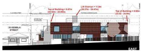
Figure 4 - Eastern elevation showing height of proposed building
