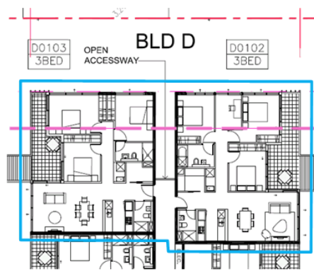
Figure 3 Approved floor plan layout of the affected units on Levels 1 and 2 in Building D (setback required to pink line)
