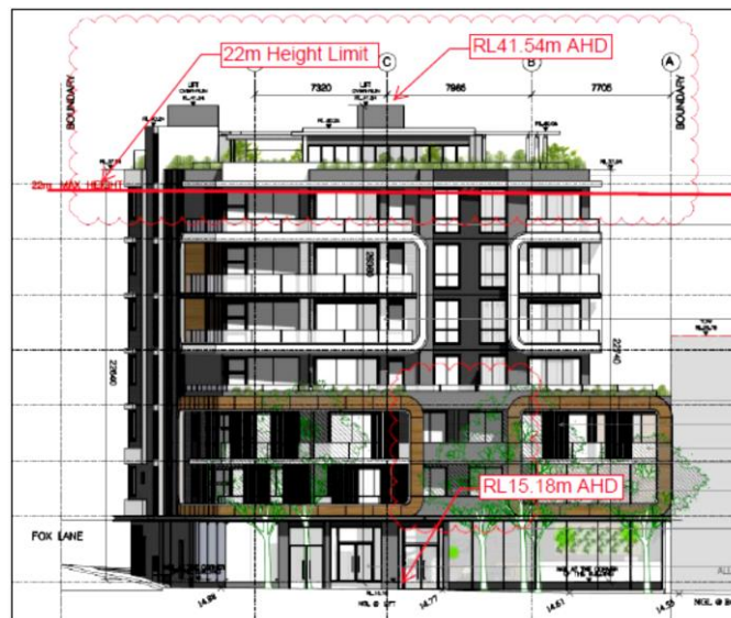
Figure 2: Extract from architectural drawing showing the maximum extent of the non-compliance with the 22m height development standard
