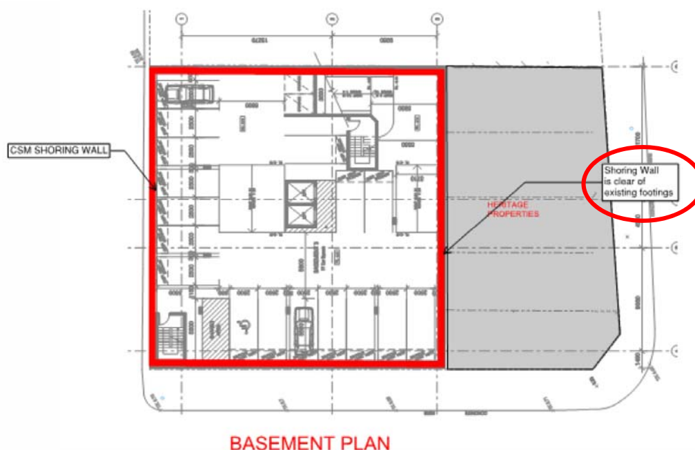
Figure 1 – Location of proposed shoring wall (Source: Structural Design Solutions, Attachment 4 )
