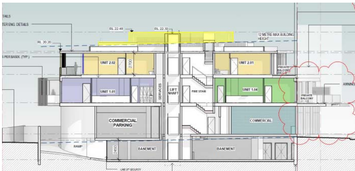
Figure 1: Section Plan demonstrating height non-compliance (highlighted in yellow)
