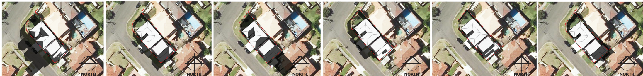
7 SHADOW - 9AM JUNE 22 1 : 500 8 SHADOW - 12 JUNE 22 1 : 500 9 SHADOW - 3PM JUNE 22 1 : 500 10 SHADOW - 9AM MAR / SEPT 22 1 : 500 11 SHADOW - 12 MAR / SEPT 22 1 : 500 12 SHADOW - 3PM MAR / SEPT 22 1 : 500
