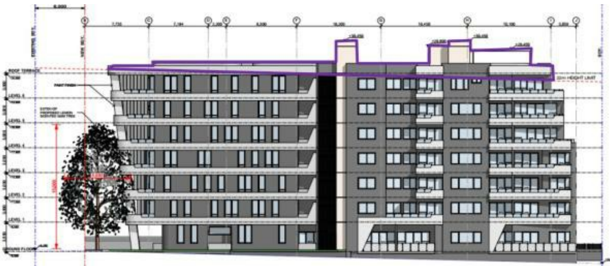
Figure 9 - Building Height exceeding maximum 22m height limit (Southern Elevation)
