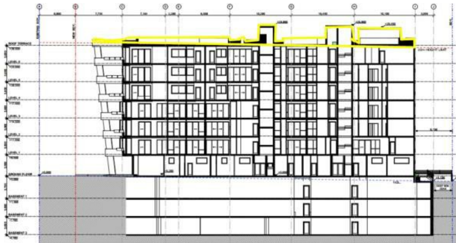
Figure 8 - Building Height exceeding maximum 22m height limit (Section B-B)
